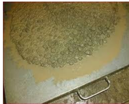
Segregation in concrete
